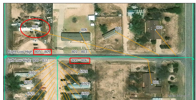
Example: Fishbone Lines - Correct (Left); Fishbone Lines - Error, due to incorrect street address range (Right)
