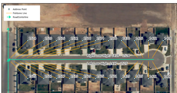
Example: Fishbone Lines - Correct (Left); Fishbone Lines - Error, due to incorrect street address range (Right)
